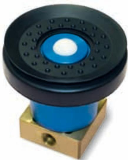
The main feature of the special built-in cups is that they open, and therefore produce vacuum, only when the load to be clamped activates the sealing ball.
