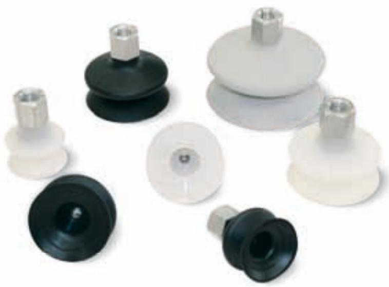
The cups described in this page, unlike the previous ones, are vulcanised onto an aluminium hexagonal support with a male or female threaded connector, inside of which there is an M8 threaded hole for the possible insertion of a calibrated grub screw (see page 1.118).
