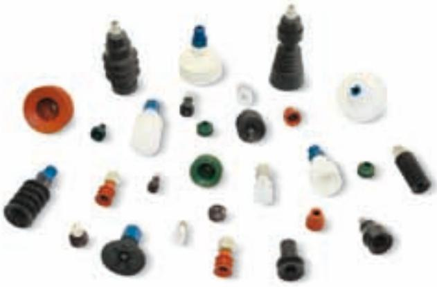
The main feature of these BELLOW CUPS is that they crumple up when in contact with surface to be gripped and in presence of a vacuum, thus creating a quick lifting movement independently from the machine. This rapid movement prevents the load beneath from remaining stuck to the lifted one.
