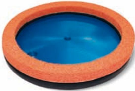
The distinctive feature of these cups is its lip made with nitrile rubber associated with GERANIUM or neoprene compounds. This allows a perfect grip on very rough or slotted surfaces. For this reason they are particularly suited for gripping and handling cement manufactures with with grit finished surfaces, marbles and bushhammered or flamed granites.
