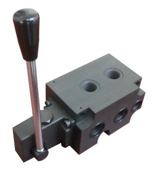
The 6/2FDV06-7... valve is manual operated flow diverter valve. It is often used to control the direction of flow for two or more double acting cylinders as shown in the connecting examples.
