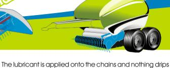
off. Lubrication takes place only when the machine is running.
