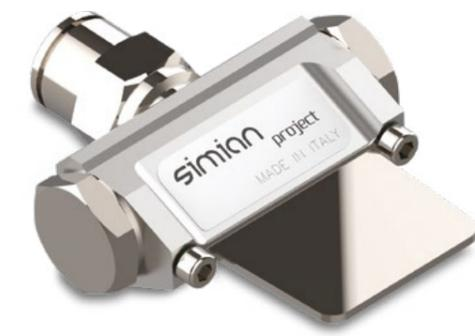
The air knives **SERIES ABT** are one of a kind, thanks to their high blowing power, which is a result of the air flow on both sides of the blade, and thanks to their easy installation, by means of two neodymium magnets and of brackets, which make it possible to direct the knife according to all demands. These products are very effective for cleaning, drying, and cooling.
