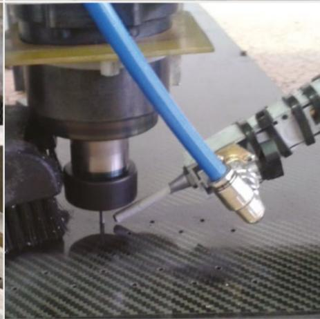
Cooler for carbon fiber's tooling
