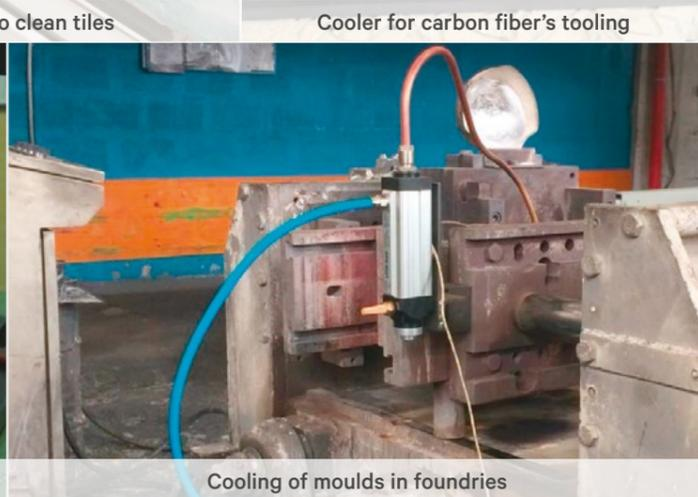
Cooling of moulds in foundries
