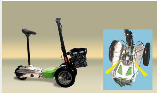
Profile dampers increase the riding comfort of an electric scooter
