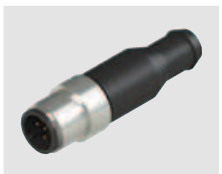
M12 terminating plugs for series connections Polyurethane connector body Protection degree IP67 Gold-plated contacts Self locking ring nut
