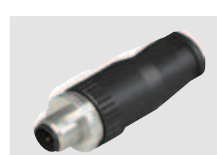
M12 plugs, field wireable Technopolymer connector body Gold-plated contacts Screw terminals for wiring Protection degree IP67
