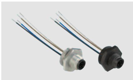
These standard M12 male connectors are ready for the installation on the switches. Their wires have the right length for the connection to the contact blocks and are provided with wire-end sleeves. On request they can be delivered already wired to the switch. The connectors are used where a very short machine down time is required (e.g. in big plants). The connector-provided switch can be replaced very quickly with an identical one with no chance of incorrect wiring.
