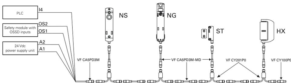
**Attention!** For proper operation of the devices connected in series via cables, Y connectors or junction boxes, it is necessary to pay particular attention to the voltage drop that occurs in the circuit. Pay particular attention to the flowing currents and cross-section/length of the used cables to ensure that the supply voltage of the components at the end of the series connection remains within the specified limit values during effective operation.
