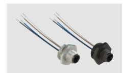
These standard M12 male connectors are ready for the installation on the switches. Their wires have the right length for the connection to the contact blocks and are provided with wire-end sleeves. On request they can be delivered already wired to the switch. The connectors are used where a very short machine down time is required (e.g. in big plants). The connector-provided switch can be replaced very quickly with an identical one with no chance of incorrect wiring.
