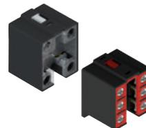
Contact blocks with captive screws, finger protection, twin bridge contacts and double interruption for higher contact reliability. They are available in multiple variants with shifted activation travels, simultaneous or overlapping. They are suitable for many different applications.
