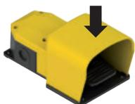
Foot switches of the PX series are provided with a reinforced shaped cap. This solution enables the cap to bear static loads of up to 800 N without breaking, therefore being tread-proof. For particularly difficult environments, the cap can be provided in material reinforced with charges in fibre glass to also resist impacts from dynamic knocks. Furthermore, for PA series foot switches in heavy duty environments it is
