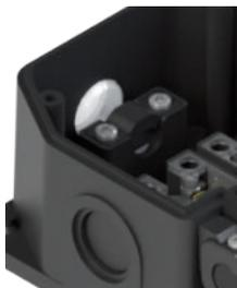
Inside the housing immediately after the cable inlet there is a cable clamp in line with the hole. Ideal for maintaining the electrical cable in position; it prevents any tractions or repeated movements from discharging on the electrical connections of the contact blocks. Reversible, it can tighten both large and small cables.
