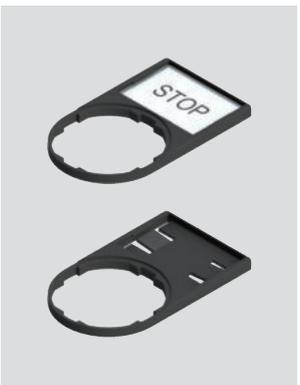
Label holders for single device, adjustable by 90° in 90° increments. The switch labels of other manufacturers can be used (for example: 3M article KE-7270-2691-3 or GRAFOPLAST article SITM612X) as long as they have the following dimensions: base 27 +0/-0.4 mm, height 18+0/-0.4 mm, thickness 0.8 ±0.4 mm.
