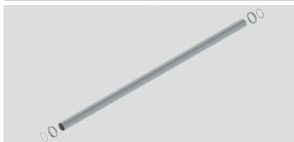
Ø 25 mm metal tube set with M25x1.5 threaded ends (for VF KIT32, VF KIT33, VF KIT34, VF KIT35) with metal nuts and gaskets. Protection degree IP65.
