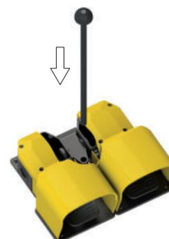
Besides the possibility of joining from two to four single foot switches, the joining elements make it possible to apply a metal tube that enables the electrical connection between the foot contacts and the contacts of an emergency push button, connected to the same tube, preserving thus an IP65 protection degree.
