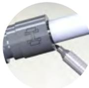
**4. MARK.** Mark the pipe at the end of the fitting for visual control (after pressing).
