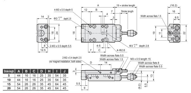
• With magnet and cylinder switch (piping direction: -R)
