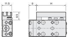
• With magnet and cylinder switch (piping direction: -L)
