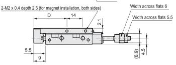
• With magnet and cylinder switch (piping direction: -R)
