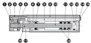
●LCM-4.5 to 8-F-P73 with magnet and switch rail
