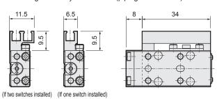
• With magnet and cylinder switch (piping direction: -L)
