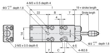
• With magnet and cylinder switch (piping direction: -L)
