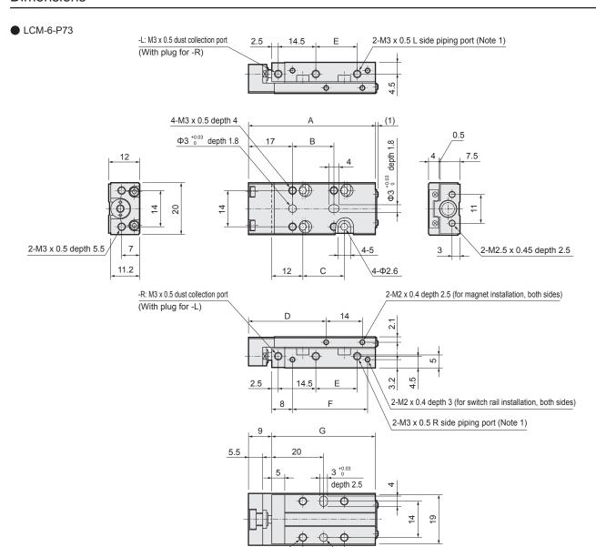
• With magnet and cylinder switch (piping direction: -R)
