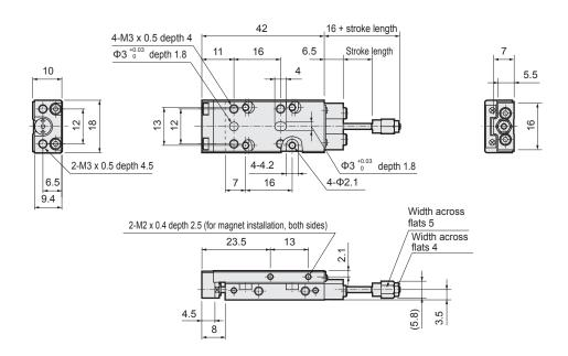
• With magnet and cylinder switch (piping direction: -R)
