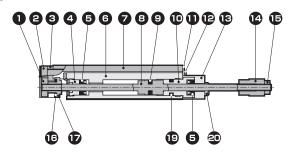
■ LCM-P-4.5 to 8 with magnet and switch rail
