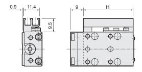
• With magnet and cylinder switch (piping direction: -L)
