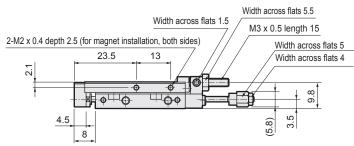
• With magnet and cylinder switch (piping direction: -R)
