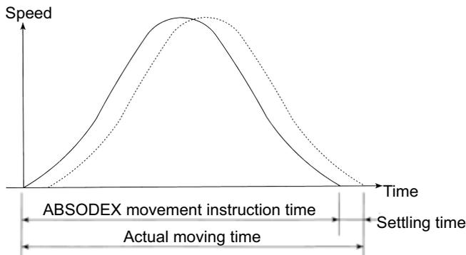
Though the stabilization time depends on working conditions, it is approximately between 0.025 and 0.2 seconds.
