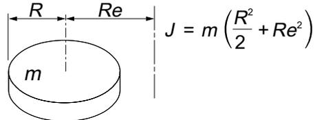
3. Hollow circular plate (hollow cylinder)
