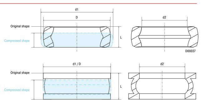
The damping elements in flange style (D00018/D00038) can apply a force or depending on the stroke can be double layer without the need for an additional spacer washer.
