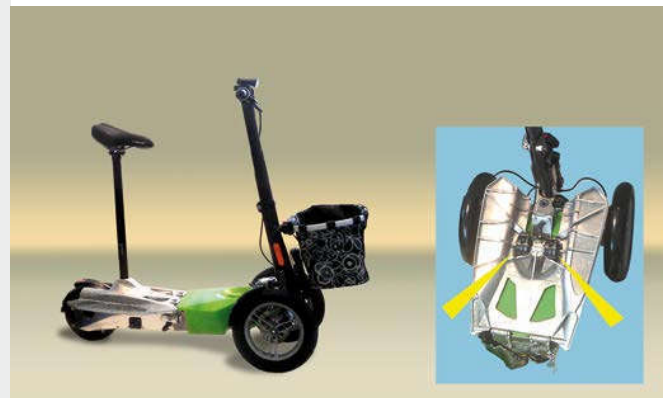
Profile dampers increase the riding comfort of an electric scooter
