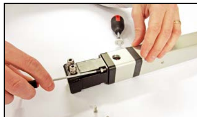
Tighten motor mounting screws
