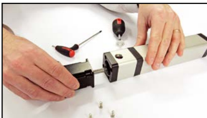
Insert motor shaft into coupling
