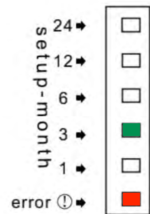
Dia. 9.2 Overloading warning (blockage)
