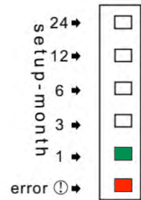
Dia. 9.1 No motor pulse warning (low battery)
