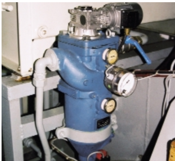
Automatic filter with internal pressure segment cleaning for engine oil in marine application
