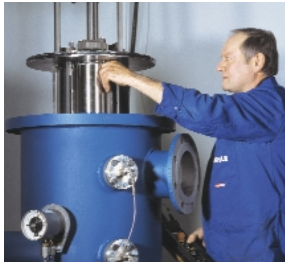
Final assembly of specially-manufactured MAHLE automatic filters
