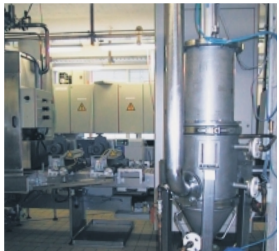
Automatic Metal Edge filter with scraper cleaning for chocolate
