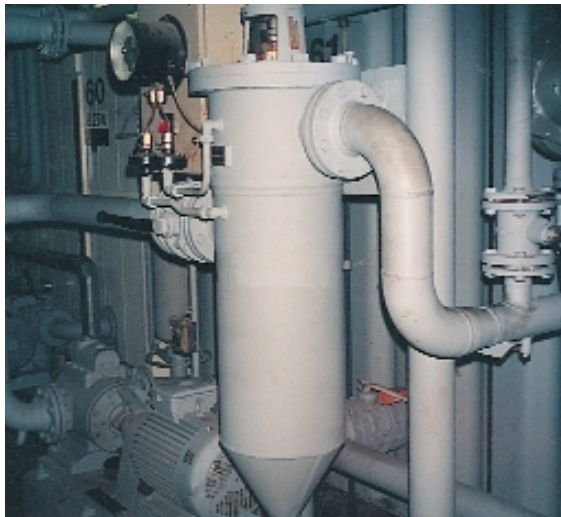
Automatic Metal Edge filter with scraper cleaning for isocyanate (a component of PU)
