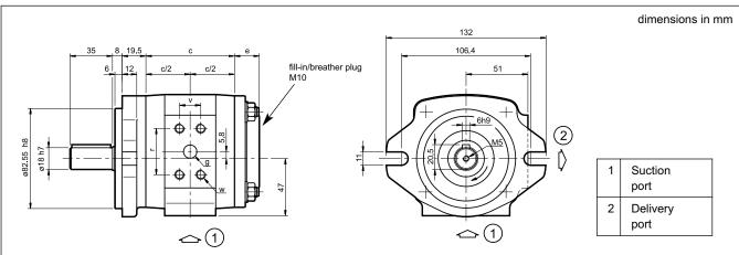
**NOTE**: the pump is shown in the clockwise rotation configuration For the counterclockwise configuration, the delivery port (2) is on the opposite side of the pump
