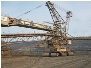
Spreader ZPDH 6300.1-CZ 342 lubrication points
