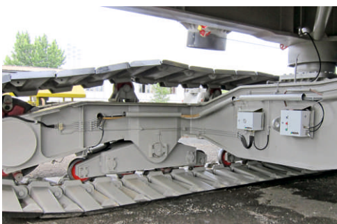
Lubrication system at the excavator's chassis
