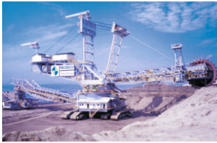
Excavator SchRs 1320/4x30 653 lubrication points
