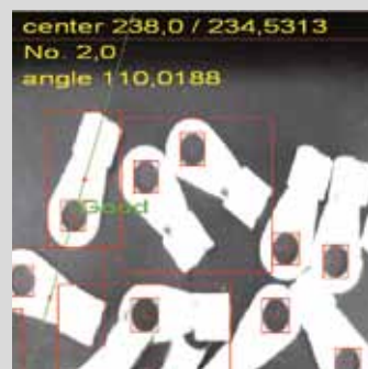
Providing direction: The correct alignment of an object is an important prerequisite for downstream processes, e.g. for positioning and tracking a gripper. Colours, shapes and contours are suitable for monitoring correct orientation.
