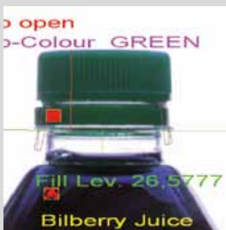
Preventing faults: Very different features can be checked at a glance with the Eyesight – here, for example, the position and colour of the cap, filling level and presence of the use-by date. This pays, because each unnoticed fault may be expensive later.
