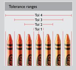
The detection window can be adapted by adjusting colour selectivity.
