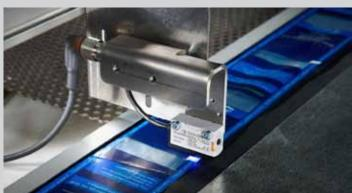
**Out with the old, in with the new:** The contrast sensors from the F 25 series are assembly and connection compatible with the conventional standard housing (image on the left). The fastening bores are aligned in the same distance from each other. The integrated cable with a M12-connector fits to the corresponding mating connector.
