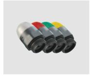
These signalling lights with high luminosity LEDs are used for signalling that an electric contact has changed its state inside the switch. They can be installed only on switches of the FL, FX, FZ, FW, FG, NG or FS series by screwing them on one of the conduit entries not used for electric cables. They can be used for many different purposes: for example, in combination with a rope switch (e.g. FL 1878-M2) they can be used to signal (even from a distance) if the switch has been actuated.
