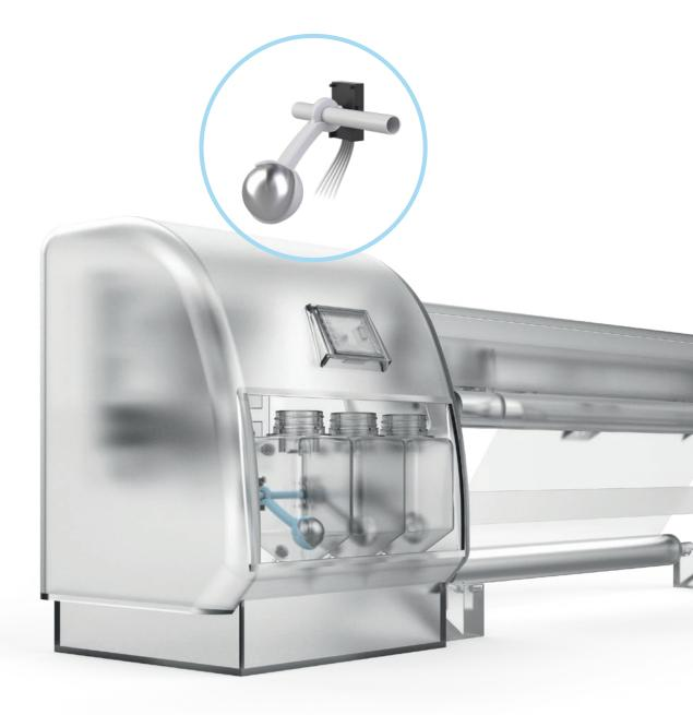
The plotter shows a sensor that was developed for industrial inkjet printers. The challenge here was to achieve an exact analogue measurement without an additional opening for the sensor in the container. The solution was the combination of a Hall element located outside of the tank with a float-magnet system in the tank.
