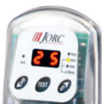
Visual display of current operating cycle
