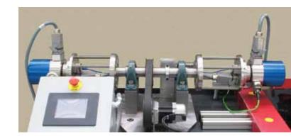
DEUBLIN slip rings undergoing life cycle tests
