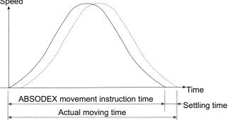
Though the stabilization time depends on working conditions, it is approximately between 0.025 and 0.2 seconds. For the travel time t1 in model selection, use the directive travel time of ABSODEX. Also, for setting the travel time with an NC program, use the directive travel time of ABSODEX.
