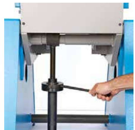
Inclination adjustment (hydraulic on 45 and 80T)
