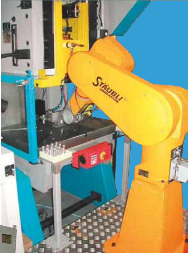
25 T press with automatic robotic loading
