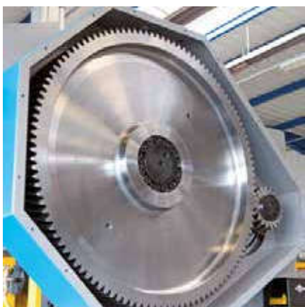
View of the 80T sprocket pinion assembly
