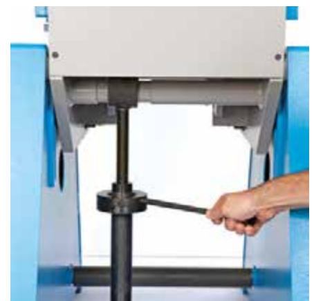
Inclination adjustment (hydraulic on 45 and 80T)
