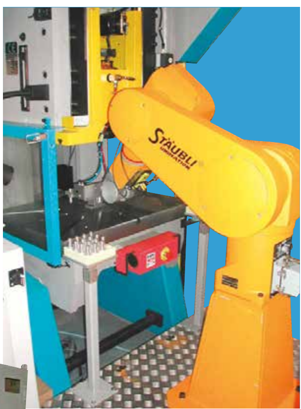
25 T press with automatic robotic loading
