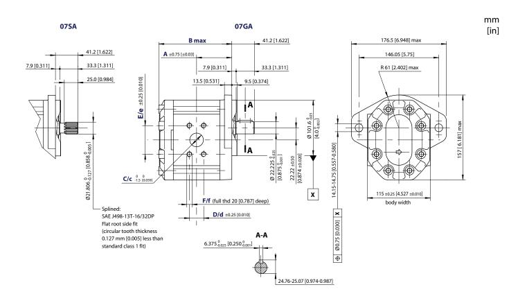
The SEP3NN overall length is 12 mm [0.472 in] less than the SNP3NN for the whole range of displacements (22.1 to 44.1 cm3/rev [1.35 to 2.69 in3/rev]).
