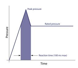
**System pressure** is the differential of pressure between the outlet and inlet ports. It is a dominant operating variable affecting hydraulic unit life. High system pressure, resulting from high load, reduces expected life. System pressure must remain at, or below, rated pressure during normal operation to achieve expected life.
