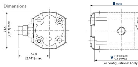
For configuration **06** (SAE A-A) dimension **B** and **V** have to be increased 4.5 mm [0.177 in].
