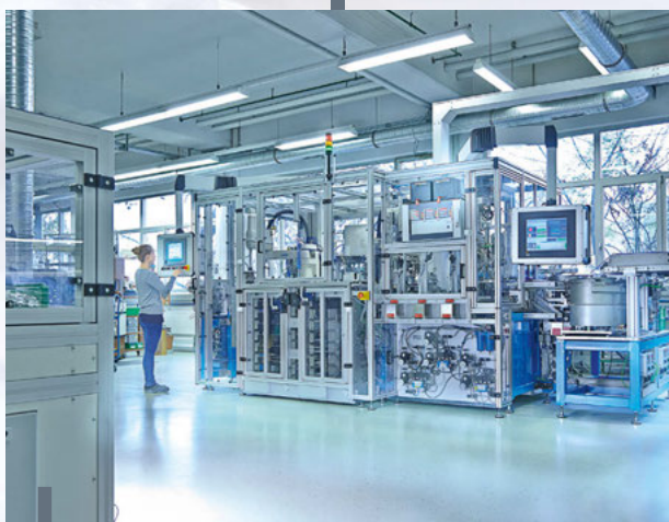
Assembly and test of pressure switches on semi and fully automated installations.
