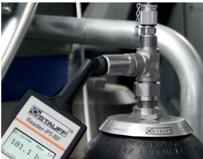
Bladder accumulator in use with Reader-PT-RF
