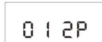
Dia. 23.5 Setting of 2P - Impulse cycles
