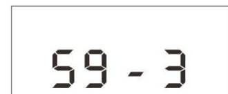
Dia. 23.7 Setting of 3P - Lube Time in Second
