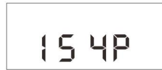
Dia. 24.1 Setting of 4P - Low Temperature
