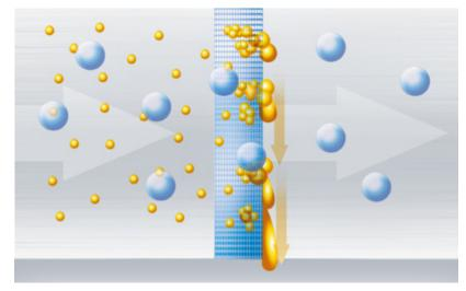
Higher performance, longer service life, and lower maintenance costs thanks to the coalescer filter principle: the oil mist "coalesces" into larger droplets, which are efficiently separated.
