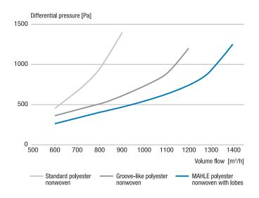
Clear performance advantage using the ridges technology: greater volume flow at a lower differential pressure.
