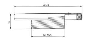
Rd72x5 adapter for installation on the clean side
