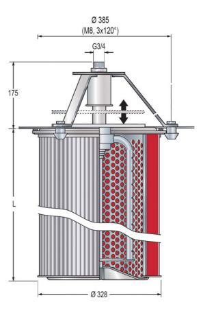
Installation on the untreated gas side A hole with a diameter of 210 mm must be drilled in the filter plate.
