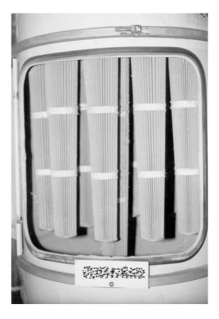
After changing to conical filter cartridges and 4,600 working hours.. Cartridges cleaned over the whole length.
