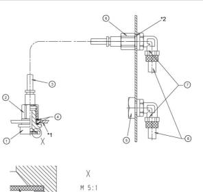
\*1 = bore Ø 13.5 mm in the filter plate \*2 = bore 2x Ø 14 mm in the housing
