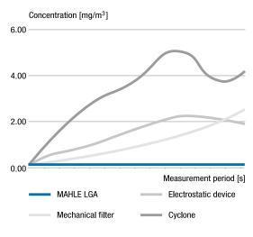
Low emissions values substantiate the consistently high retention efficiency of the MAHLE LGA series (in comparison with conventional separators).
