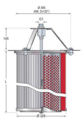
Installation on the untreated gas side
