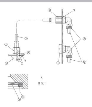
\*1 = bore Ø 13.5 mm in the filter plate \*2 = bore 2x Ø 14 mm in the housing
