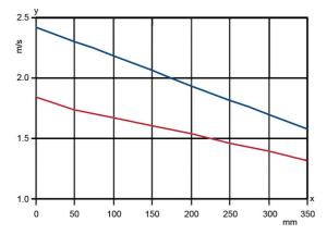
The conical design of the cartridge shows a high reduction of the upstream velocity in the area of the bottom end cap. Through it the element is much better to clean off, especially in use of light dust. The dust can sediment better.
