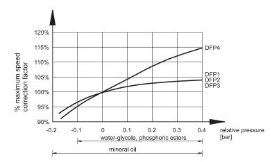
If the pressure in the suction line is different than zero, the maximum rotation speed shown in table 3 must be multiplied by the correction factor obtained from the diagram seen on the left.
