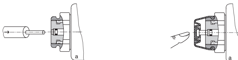
Basic versions of the manual override using pin or push button placed in the protective rubber sleeve.
