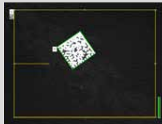
Code reading on solar cells Even extremely small codes (e.g. on silicon solar cells) or highly reflective codes (e.g. on thin-layer solar cells) can be read.
