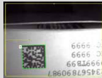
Printed codes on pharmaceutical packaging ECC200 or bar codes (e.g. EAN 13) can be searched for simultaneously. In addition to code reading, the presence of optical characters can also be checked using object detection.
