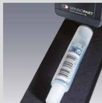
Printed data matrix code for identification of pharmaceuticals
