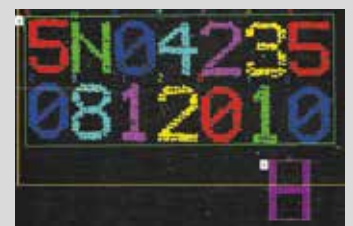
Lasered data matrix code for identification of plastic components
