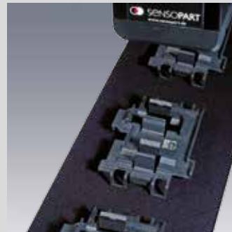
Lasered data matrix code for identification of plastic components
