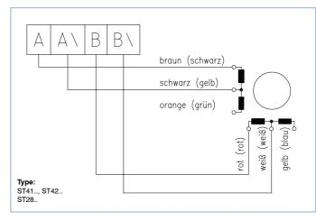
Current per winding x 0.7 = current per phase Example: Current/winding 1A = 0.7A/phase
